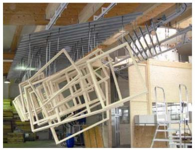
Caption: The Power & Free system of Conductix-Wampfler is used, among other things, in coating plants for wooden window-frames. Minimal space is needed due to transverse buffering.
